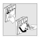
You can thus clean it using running water and a brush or a twisted cloth. Check that the siphons at the back of the detergents dispenser are not blocked.
